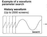
Detects waveforms whose specified waveform parameter exceeds a specified range.
