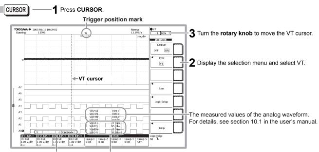
T: The time from the trigger position to the cursor position
