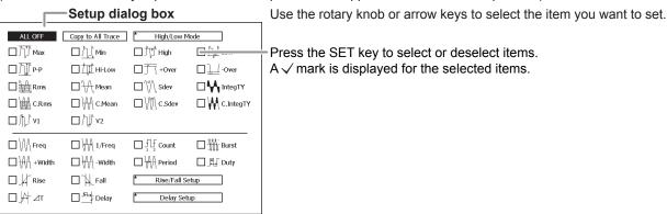
(When these soft keys in the setup menu are pressed while the setup dialog box above is displayed: Area/Calc > Calc)
