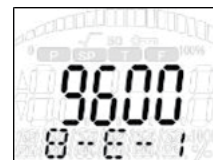
Serial information (3 s) E.g.: Baud rate: 9600 [bps] Data Length: 8 [bit] Parity: Even Stop Bit: 1
