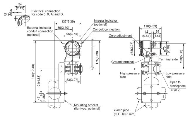
\*1: When electrical connection code 7 or C is selected, a blind plug is protruded up to 8 mm from the conduit connection.
