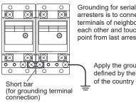
Grounding for serial installation of arresters is to connect grounding terminals of neighboring arresters to each other and touch ground at one point from last arrester according.
