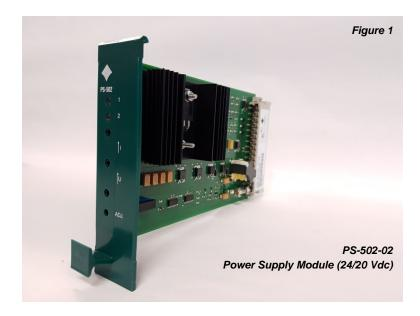
The module converts the 24 V field voltage into a galvanically isolated and regulated 20 V logic voltage.
