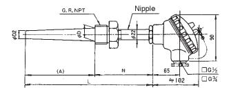
\*: Model RM-2 with the length of L-A < 50 mm is not available. Model RM-3 with the length of L-A < 60 mm is not available.
