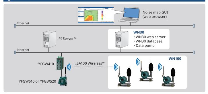
The principal components of this system are the WN100 wireless noise meter and the WN30 noise mapping software. Compliant with the ISA100 Wireless network protocol, WN100 sensors can be installed at many locations throughout a plant to measure noise levels and transmit this data in real time to servers via gateway devices such as
