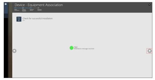
The system will look for the installation message coming from the telemetry device. Once the message is received you can then see the thermostat information: this will help you to verify if the telemetry has been properly installed.
