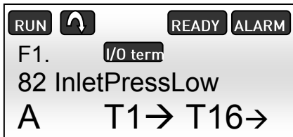
Figure 7.1-4, Low pressure alarm on the NXP panel
