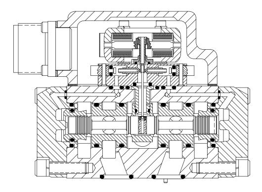
Vickers by Danfoss SM4-20 servo valves can provide system closed loop control with exact positional accuracy, repeatable velocity profiles, and predictable force or torque regulation.
