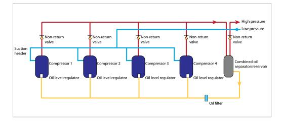
An active system can offer more flexible and efficient oil management. It is highly recommended for manifolding since this positive system increases the reliability of the manifolding configuration. Oil management will be secured mainly by the oil level regulator and the oil separator, which can supply the oil when required. The active system can thus accommodate itself to various oil conditions.
