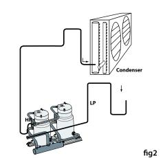
Note: Suction accumulator and Oil separator etc. are not shown in this illustration, but those are necessary for the system. The graph above is only for piping design considerations.
