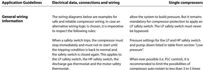
In specific situations, such as winter start operation, an eventual LP control for pumpdown cycles may be temporarily bypassed to mandatory for compressor protection to apply an LP safety switch. The LP safety switch must never
