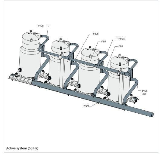
Note: The dimensions are external diameters, for quadro systems, it is necessary to add support at discharge line. Active system (50 Hz) excluding non-return valve, oil separator/reservoir and oil regulator. The compressors shown here are brazed version, but could also work with rotolock version.
