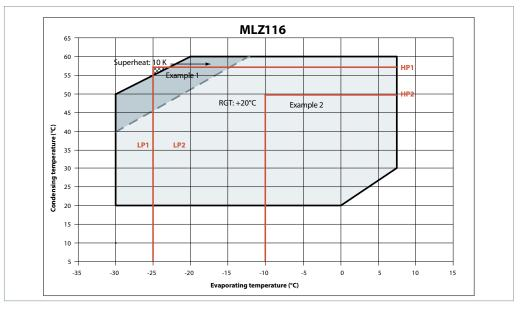
Example 1 (R22, SH = 10 K) LP switch setting: LP1 = 1 bar (g) (-25°C) HP switch setting: HP1 = 21.8 bar (g) (58°C) The LP and HP switches don't protect sufficiently from operation outside the envelope. A DGT protection is required to avoid operation in the hatched area. Example 2 (R22, SH = 10 K) LP switch setting: LP2 = 2.5 bar (g) (-10°C) HP switch setting: HP2 = 18 bar (g) (49°C) O The LP and HP switches protect from operation outside the envelope. No DGT protection required.
