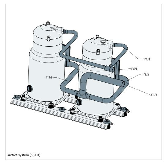
Note: The dimensions are external diameters. Active system (50 Hz) excluding non-return valve, oil separator/reservoir and oil regulator. The compressors shown here are brazed version, but could also work with rotolock version.
