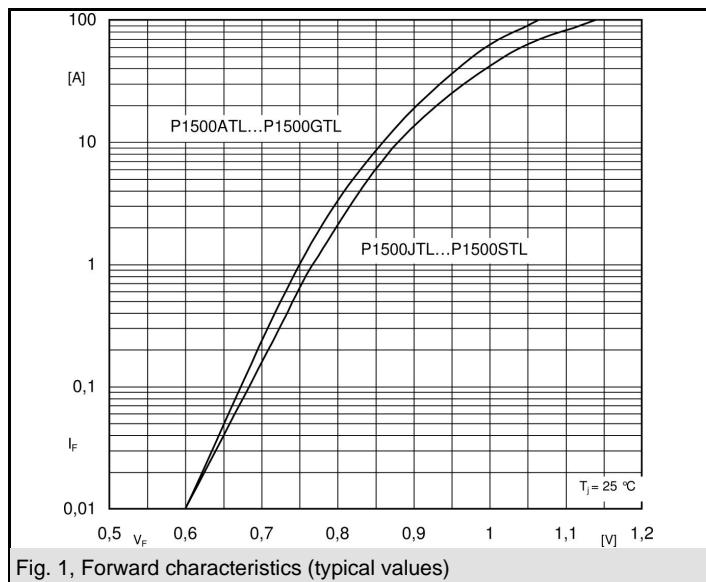
Fig. 1, Forward characteristics (typical values)
