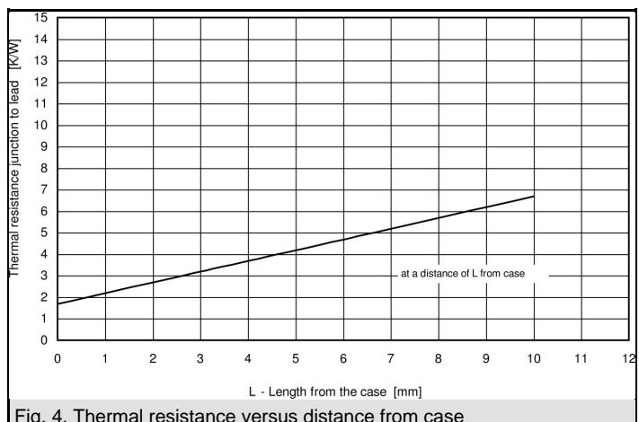
Fig. 4, Thermal resistance versus distance from case
