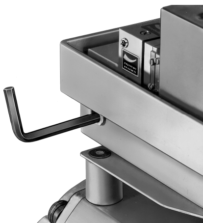
Fig. 19: Tightening feedback lever
