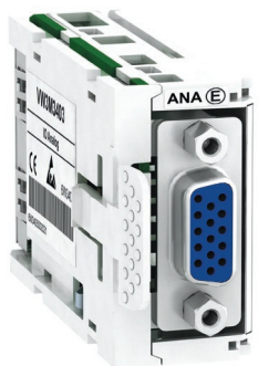
VW3M3403 encoder interface card (analog output)
