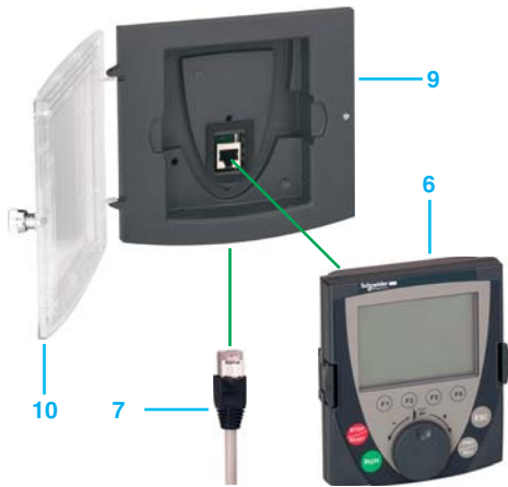
Remote location of the graphic display keypad on enclosure door: 6 + 7 + 9 if IP 54, 6 + 7 + 9 + 10 if IP 65
