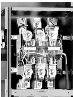
225 A Ringless-Type Meter Socket, Seven-Jaw with Lever Type Bypass Shown with Lexan Shield over Line and Load Meter Jaws
