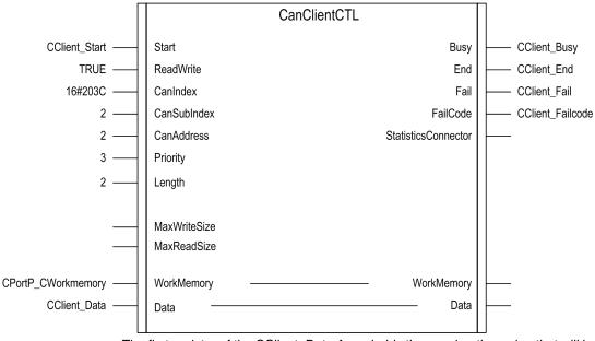
The first register of the CClient\_Data Array holds the acceleration value that will be sent to the device every time that CClient\_Start is TRUE and the CClient\_End reading operation ends in TRUE.
