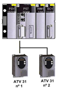
**NOTE:** This example can be applied to any CPU of the Modicon M340 and Premium families that can communicate on CANopen.
