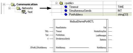
The name of the "EGtwMB\_MBWorkMemory" variable must be the same in the "ModbusClientBasic" and "ModBusGateway."
