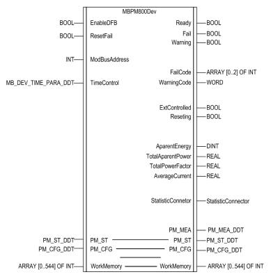
The functional module that will be used in the program has the following aspect (at the FBD block level) after PLC generation in UNITY Pro:
