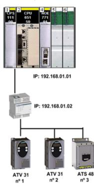
The objective is to establish communications with a Quantum PLC towards an ATS48 Modbus slave (Modbus slave number 3) through a Modbus Ethernet-Serial Modbus gateway in order to write to the cascade function activation register (register 4058).
