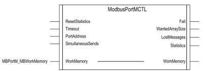
The name of the "MBPortM\_MBWorkMemory" variable must be the same in the "ModBusClientBsCTL" and "ModBusPortMCTL".
