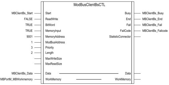
The first register of the MBClientBs\_Data[0] Array holds the acceleration value, and the second register holds the deceleration read from the device every time that MBClientBs\_Start is TRUE and the MBClient\_End reading operation ends in TRUE.
