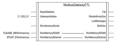
The XWAY messaging address with which communications should take place must be edited in the PLC Ethernet port configuration:
