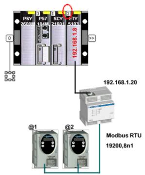
The same structure used in the previous section is used here. The objective is to establish communications with a Premium PLC towards an ATV31 Modbus slave (Modbus slave number 1) through a Modbus Ethernet-Serial Modbus gateway in order to read the Acceleration value (register 9001).
