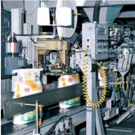
Lexium 32i integrated drive controlling a packaging line
