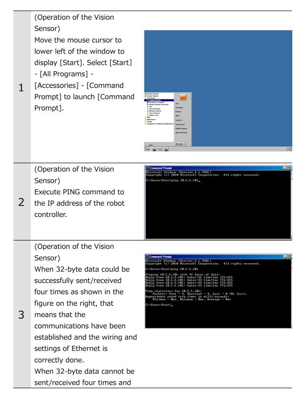
PING command timed out, check whether or not the robot controller is turned on, the wiring was correctly done, or communication settings are correct.
