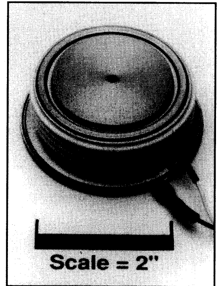
C451 Phase Control SCR 1500 Amperes Average, 2400 Volts
