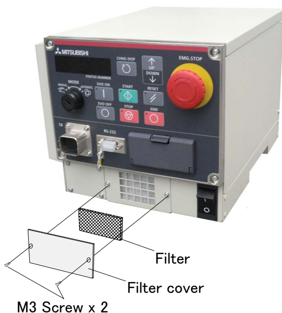
Fig. 5-3 : Cleaning, exchanging the filter(CR1DA-700)
