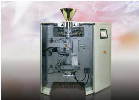
Figure 2: Tubular bag machine: The system uses predefined function blocks especially for packaging machines which can be used to set up control systems including HMIs quickly and easily.
