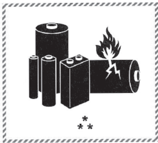
Figure 1: Lithium battery mark example
