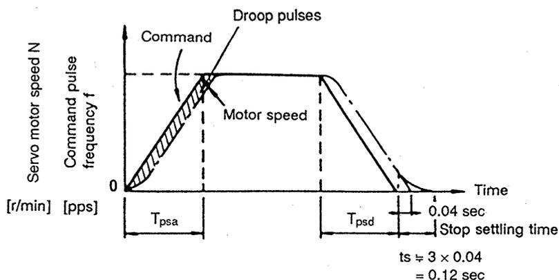
(2) Stop settling time ( $t_s$ ) during linear deceleration
