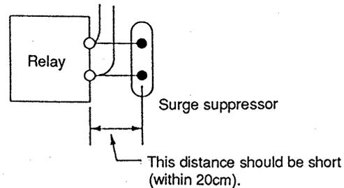
(Ex.) 972A-2003 504 11 (Made by Matsuo Electric Co., Ltd. — 200VAC rating)
