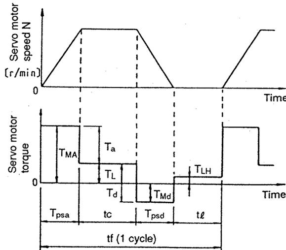
$$T_{rms} = \sqrt{\frac{T_{Ma}^2 \times T_{psa} + T_L^2 \times t_c + T_{Md}^2 \times T_{psd} + T_{LH}^2 \times t_l}{t_f}} \dots\dots\dots(7-12)$$
