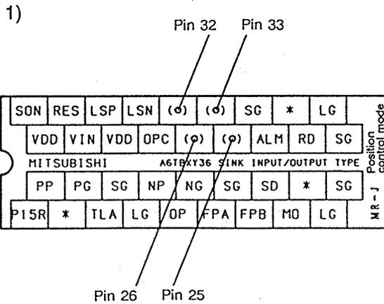
Refer to Section 3-5.5 for the setting details and explanation of the 25, 26, 32 and 33 pins in the position control mode.
