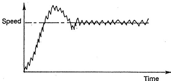
Note: The speed feedback signal (speed monitor) viewed on the oscilloscope may have ripples of short durations as shown on the left. These ripples are produced because of the PWM system used for monitor output.
