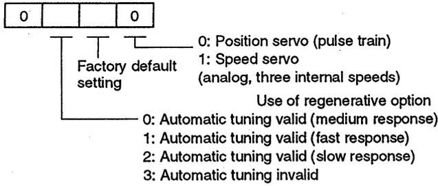
First, execute the automatic tuning with the medium response set as the factory default setting to confirm the operation.
