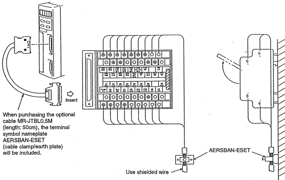
Use the AERSBAN-ESET (cable clamp /earth plate) enclosed with the cable when connecting the relay terminal block (A6TBXY36).
