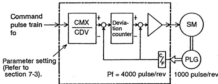
As shown above, the command pulse is multiplied by CMX/CDV to become the position control pulse. Therefore the movement amount per command pulse,  $\Delta l_o$ , is expressed with the following equation.
