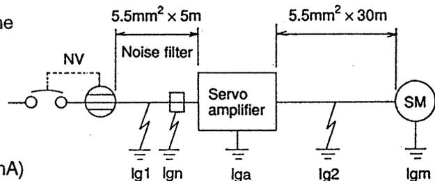
$$\text{Rated sensitivity current} \geq 10 \times \{I_{g1} + I_{gn} + I_{ga} + K \times (I_{g2} + I_{gm})\} \text{mA}$$
