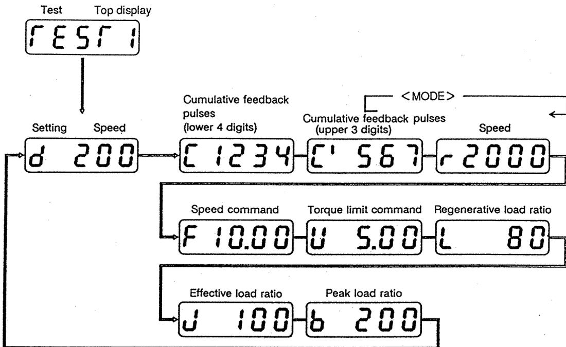
The set speed will be 200r/min when switched to the test operation screen.
