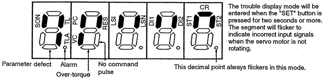
If the LED segment is flickering, the reasons for the servo motor not rotating can be determined from the following chart.
