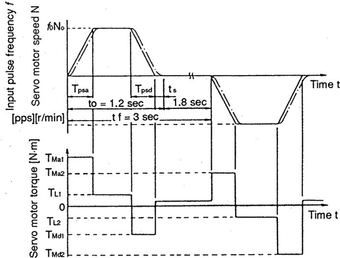
Calculate the acceleration and deceleration times required for positioning performed under the conditions of  $t_o = 1.2$  (sec) or less and  $l = 700$  (mm), shown in the figure above, as given below. To increase the stopping accuracy, determine  $t_s$  as follows.
