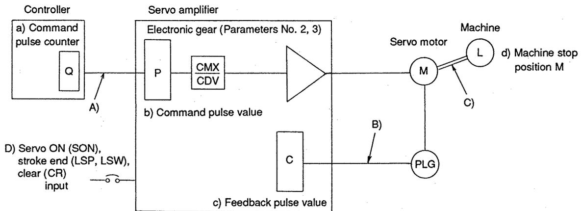
In the above diagram, (a) command pulse counter, b) command pulse value P display, c) feedback pulse value C display, and d) machine stop position M represent points to be checked when a position offset occurs.
