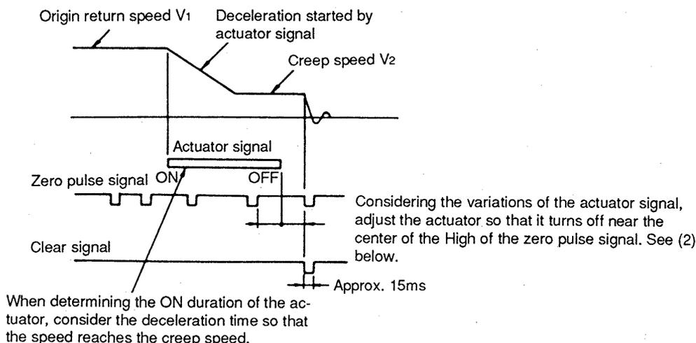
Fig. 7-1 Origin return using the actuator
