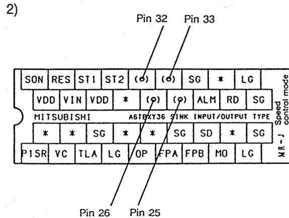
Refer to Section 4-5.5 for the setting details and explanation of the 25, 26, 32 and 33 pins in the speed control mode.
