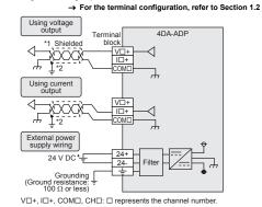
\*1 Use 2-core shielded twisted pair cable for the analog output lines, and separate the analog output lines from other power lines or inductive lines.
