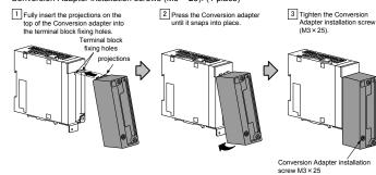
Before tightening the installation screws, check that the Conversion Adapter has been securely installed on the MELSEC-L Series module. Tightening the screws in floating-off state or tilting state will damage the Conversion Adapter installation screws and the mounting bracket
