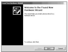
The screen shown on the left appears when you connect the personal computer and QCPU (Q mode) by the USB cable.
