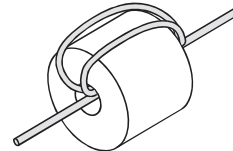
Lead through three times (three turns)
