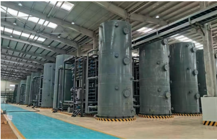
DLE is already producing lithium at industrial scale at a handful of sites. This plant in China, owned by EVE Energy Co. Ltd, extracts up to 10,000 tpa LCE (battery grade) from brines using DLE technology provided by Sunresin New Materials Co. Ltd. The lithium concentration in the brine which is treated at this plant is 100-120 mg/L (Photo: Sunresin New Materials Co. Ltd).
