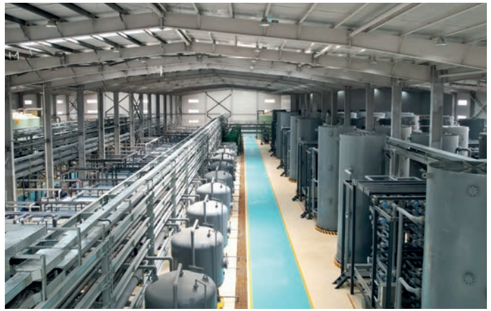
DLE is already producing lithium at industrial scale at a handful of sites. This plant in China, owned by EVE Energy Co. Ltd, extracts up to 10,000 tpa LCE (battery grade) from brines using DLE technology provided by Sunresin New Materials Co. Ltd. The lithium concentration in the brine which is treated at this plant is 100-120 mg/L (Photo: Sunresin New Materials Co. Ltd).
