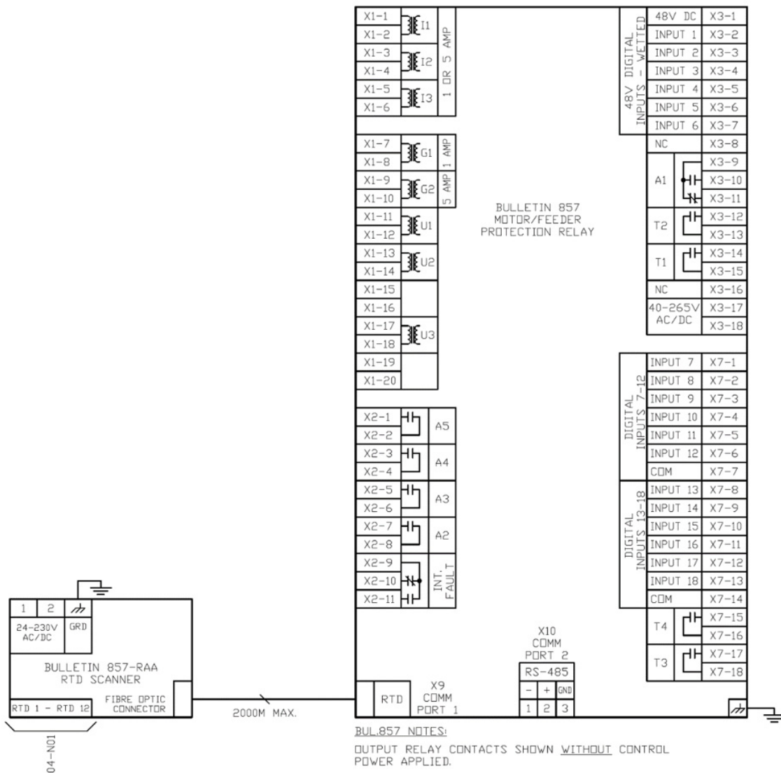
Typical Bulletin 857 Relay Electrical Diagram with RTD Scanner
