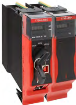
GuardLogix 5580 Controller with Safety Partner
