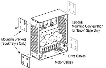
**3.** Use the figure below or an actual unit to mark the mounting holes. Drill and tap the four (4) device mounting holes.
