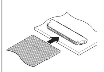
The large miniaturization at pitch direction and depth direction and low profile as 1.2 mm mounting height are realized. FH connector is miniaturized and space saving Non-ZIF type connector for FPC.
