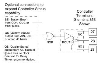
The controller status output contact can be used to activate one or more of the following alarm annunciators.
