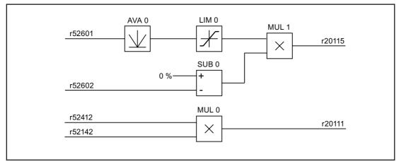
r52601 Speed setpoint behind ramp-function generator of drive 1 via peer-to-peer word 1
