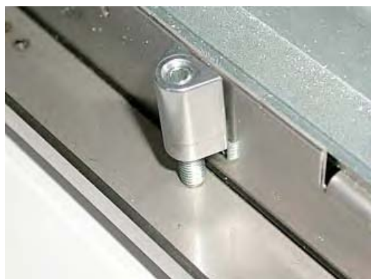
Figure 5-4 Proper positioning of the clamp
