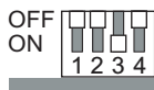
Figure 5-34 Settings on the 4-pin DIL switch to reset the integrated MD4 modem
