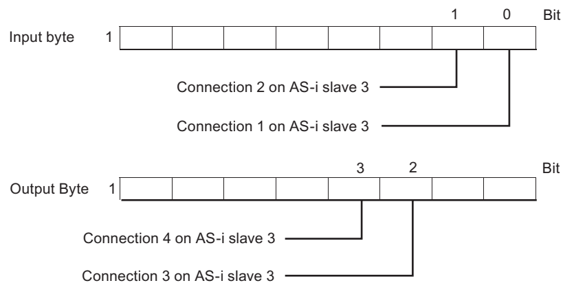
Figure 5-10 Assignment of the AS-i connections of the AS-i slaves to the data bits of the input/output bytes
