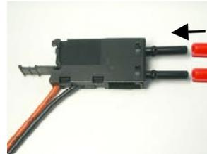
A black connector adapter is shown with two red dust protection caps being pushed onto the fiber optic cables. An arrow points to the left, indicating the direction of movement. |
