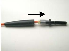
A black anti-kink sleeve is being pushed onto the end of a fiber optic cable. An arrow points to the right, indicating the direction of movement. |
