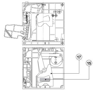
Mount the fixing plate (16) on the circuit-breaker cover and fix it with the screws (10) and (12) (see preliminary operations).
