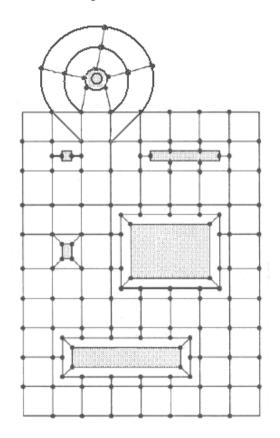
The following figures show examples of a suitable layout for a structural joint (1):
