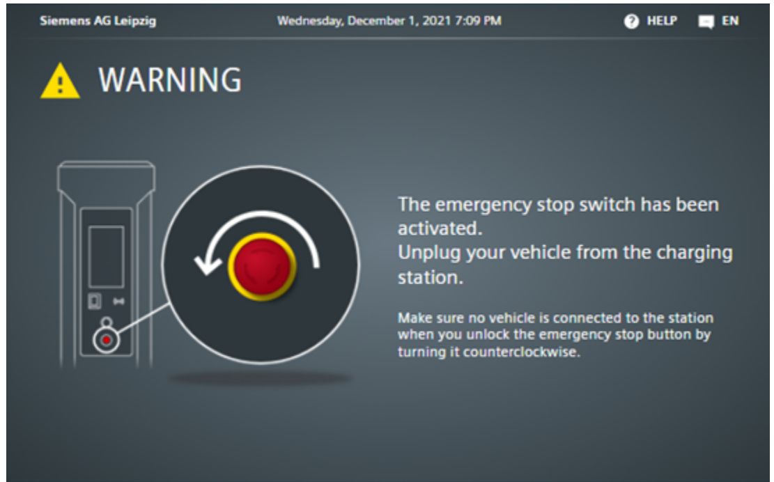
Figure 8-1 Error message "The emergency stop switch has been activated"
