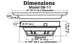
**Note:** The Model DB-11E base detector has a diameter dimension of 4.5" (11.4 cm).
