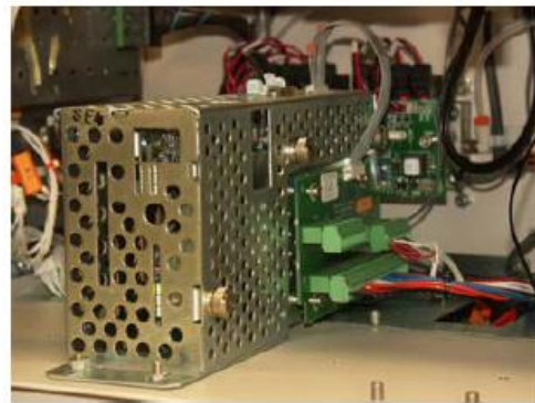
Figure 3. SNE Enclosed Housing with DPM Connector Board
