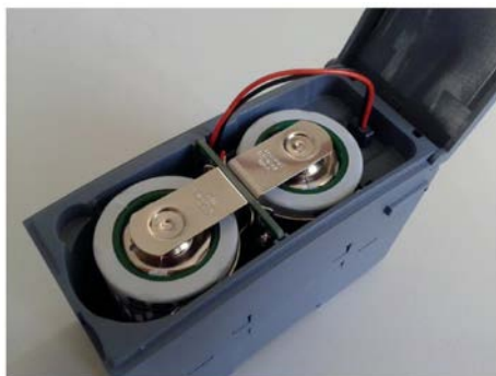
Figure 3-10 Battery module (not mounted) with inserted battery holder, cable connected.
