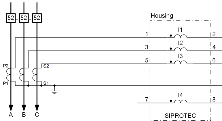
Current transformer 3-phase: connection = 3-phase
