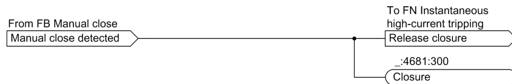
Figure 5-23 Logic Diagram of the Closure-Detection Function Block
