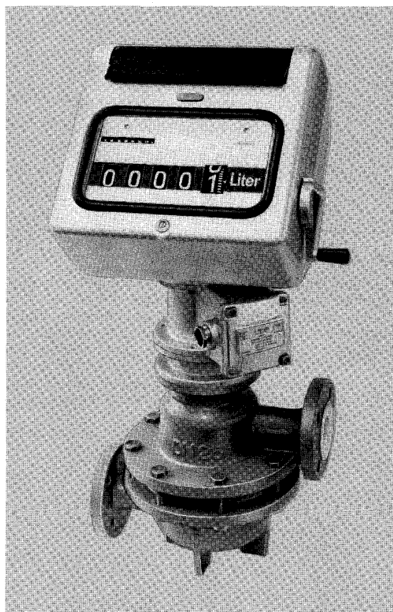
Fig. 1/3 Rotary-piston meter of enamel/plastic design DN 25 with resettable drum-type counter with ticket printer type 22 and pulser
