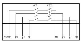
A floating signal (4x NO) is available on the Ex p control unit. This signal can either be used as an enable that is also safety related. Or it can be used as a floating signal.
