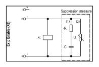
This circuit variant is used for inductive loads AC voltage fed relays / contactors. In this circuit variant, the property of the VDR resistor is exploited to become low-resistance above a certain threshold voltage. This short-circuits the self-induction voltage.
