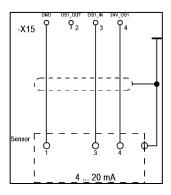
Pressure or gas sensors with 4...20 mA output can be connected to the sensor input OS 1 [Ex ib].
