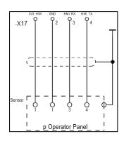
The optionally available p operator panel can be connected to the terminal row "X17".
