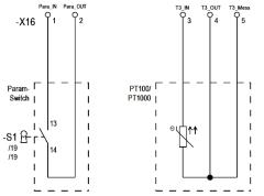
The BARTEC parameter-setting switch must be used to change the parameters.
