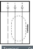
The supply voltage is connected to terminal row X3.
