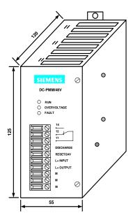
Abmessungen / Dimensions: 125 mm x 120 mm x 55 mm
