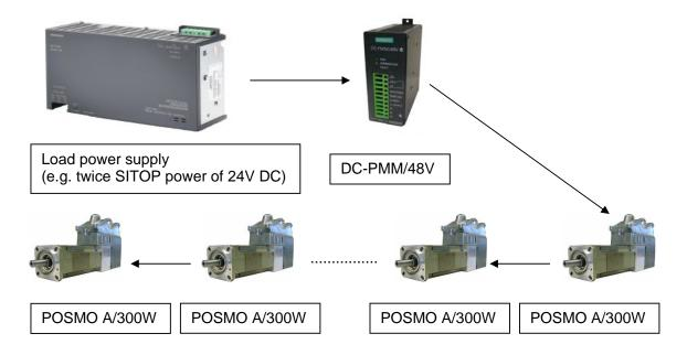
The DC-PMM/48V is connected directly after the load power supply and before the first POSMO A, with terminals L+ Input and M (existing three times altogether) of the PMM to be wired to the load power supply, terminals L+ Output and M to be wired to the first motor
