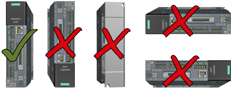
Figure 5-1 Converter mounting orientation
